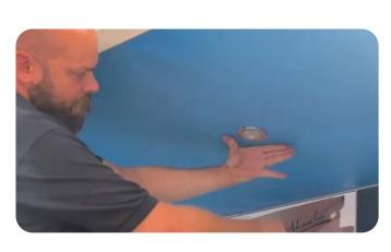
The clip will spring back once fitted through the designated hole, holding the light in place.
